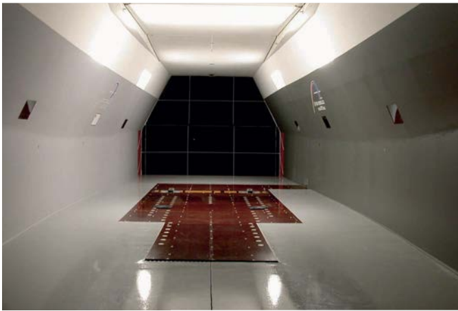
Wheels are not rotated in A2, the smaller alternative to the main tunnel
